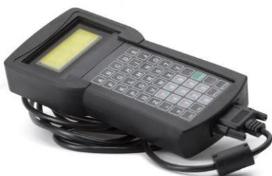
A hand held alphanumeric LCD remote control is included. The device is needed for smoke samplings, but can also be used in gas samplings, for entering useful vehicle info to analyzer, and for guiding operator to specific test modes.
